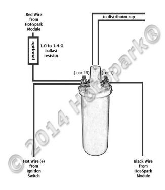
**Test Maximum Charging System Voltage**: If the charging system voltage, measured at the coil's positive terminal, is more than 14.0 volts at any RPM level, the voltage regulator likely needs replacing. Too much voltage can damage the coil, ignition module and other electronic components. A maximum charging system voltage of 13.7 volts or so is plenty. A quick fix would be to wire an external ballast resistor between the coil's + terminal and the HotSpark ignition's red wire.
